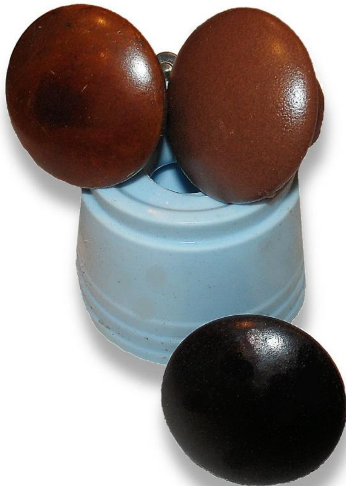
The original and two copies of a wooden bureau knob along with the silicone mold. One copy was created using KastEZ resin for the oak finish, the other with AquaClear resin for a mahogany look.
