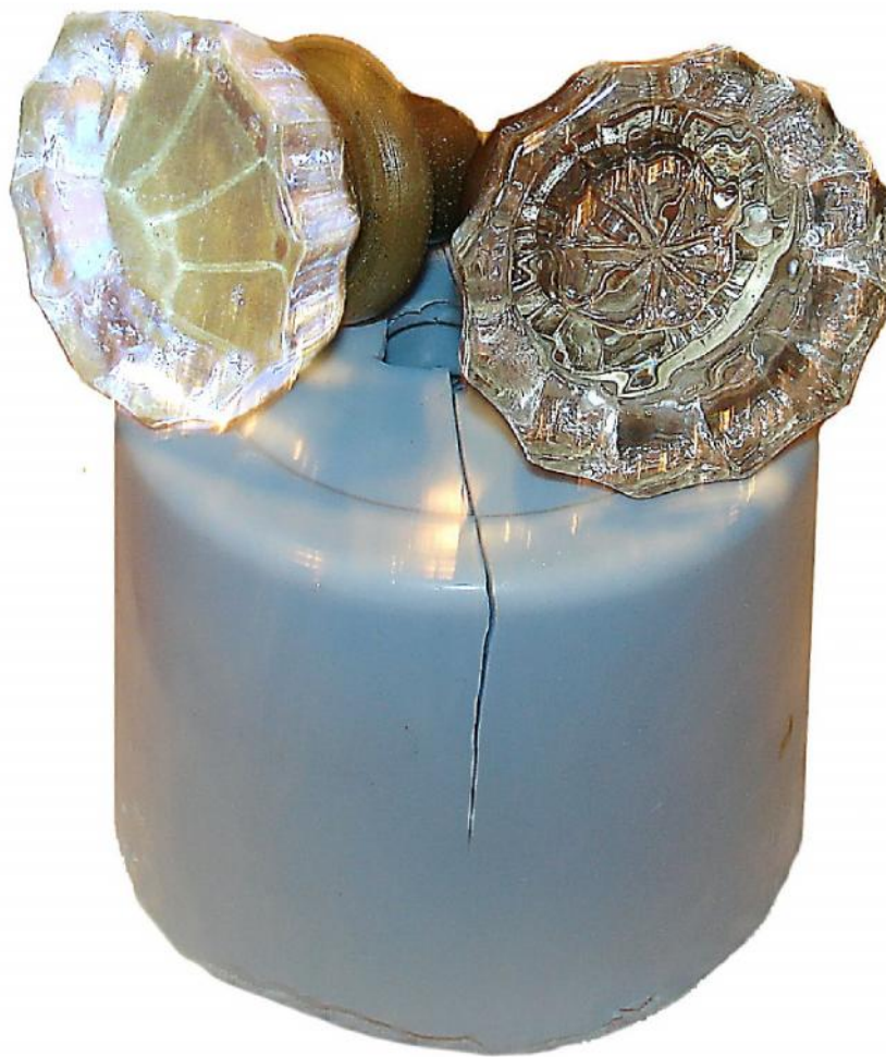
The duplicate glass knob along with the original sitting on its mold of MoldRite25 RTV silicone rubber.
