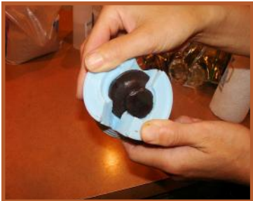
The mold is vibrated as the material sets. Once set, the mold is opened to reveal the finished duplicated knob.
