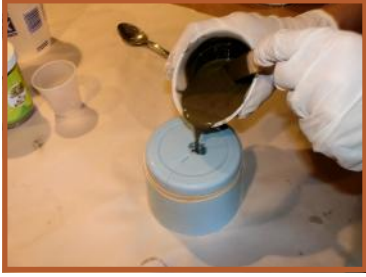
After mixing 1/3 dry pecan shell powder with 1/3 Part A and 1/3 Part B of resin, the mixture is poured into the mold.
