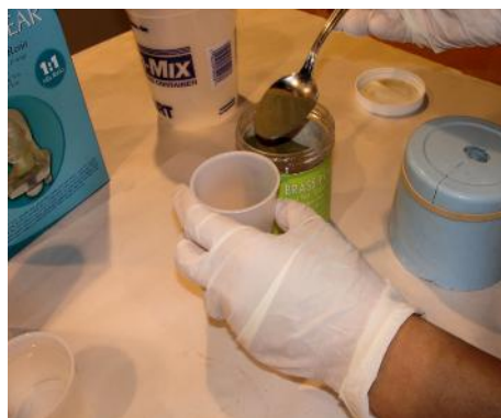
Step 13. We then spooned out brass powder in a third cup to the same level we measured for Part A and Part B of AquaClear resin.
