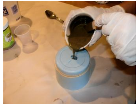
We filled the mold with the mixed brass casting material all the way to the mold opening. We then vibrated the casing until it set.
