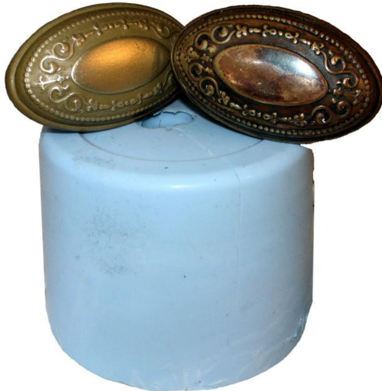
The duplicated brass knob is on the left. The original is on the right. The original still has a worn lacquer surface which adds to its antique look. In time the duplicate will oxidize to a similar patina.
