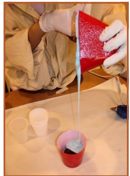
MoldRite 25 is mixed and pour on top of the knob to create the mold.
