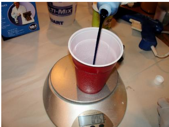
Step 5. In a separate cup we measured out Part B of MoldRite 25 Part B is 1/10 the weight of Part A. We almost forget to account for the weight of the cup. By placing the empty cup on the scale and pressing the 'tare' button the scale automatically set itself zero and the weight of the cup was then accounted for. We measured out 10 grams of Part A and 1 gram of Part B.
