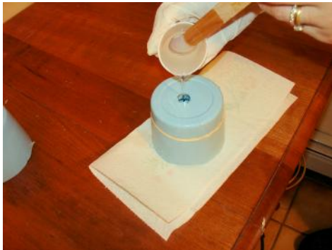
We created a door knob mold using the method on the previous pages. AquaClear resin was mixed and poured to the level of the glass door knob being careful not to fill above the line where the brass connects. Then we vibrated
