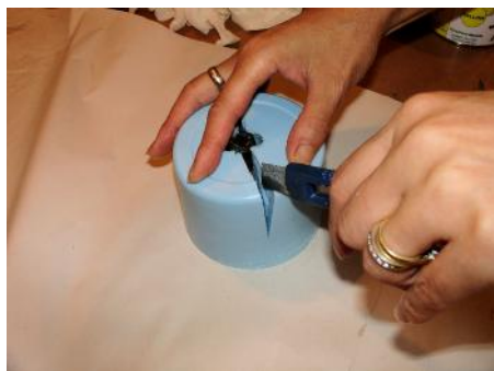
Step 8. When the mold rubber has set, we sliced open the mold with a razor or X-Acto knife. We cut opposite sides and 2/3rds of the way down .
