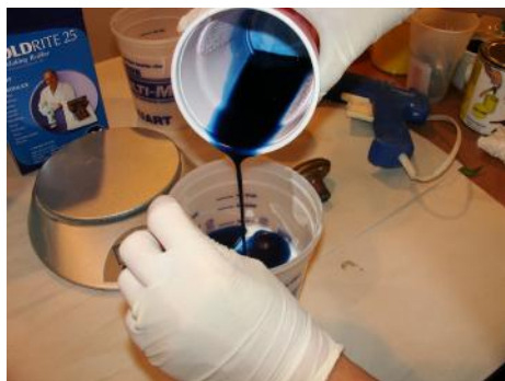
Step 6. Once Part A and B are measured combine the two parts and mix until you have an even color with out any marbling.
