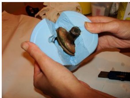
Step 9. The mold was spread open the like a clam shell to remove the original part.
