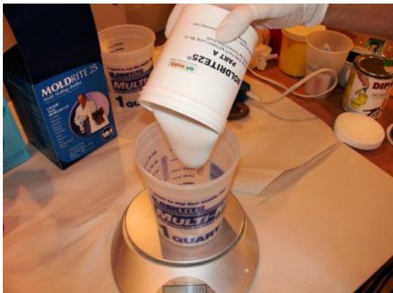
Step 4. We measured out Part A of the MoldRite 25 using the gram scale. We wanted enough material to cover our knob about 1/2-inch higher than the highest point. Since we were using the same container as our mold box to pour in Part A it was a simple matter of filling the empty container to the same level mark that would equal 1/2-inch above the knob. Once filled to the correct level we noted the weight.
