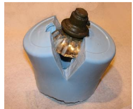
After the brass cast was set we removed knob from the mold and cleaned up the flashing. And polished the brass with 000 steel wool.
