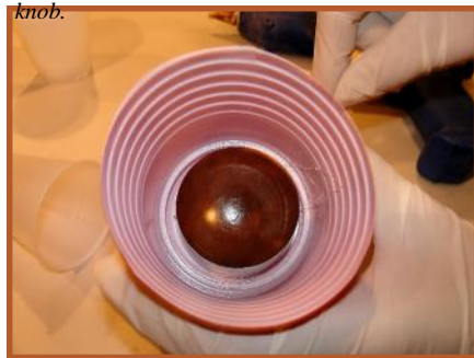
The knob was secured to the bottom of a mold container. Here we used a cut off plastic cup.
