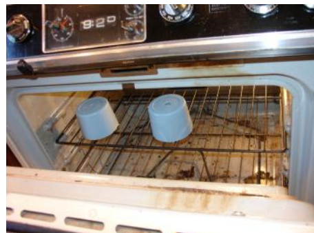
Step 10. The mold was baked in the oven at 150-200 F° to outgas any residual alcohol remaining in the mold.
