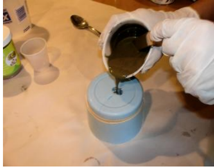
Step 15. Part A and Part B was combined in a separate cup and thoroughly mixed before it was poured into the mold.
