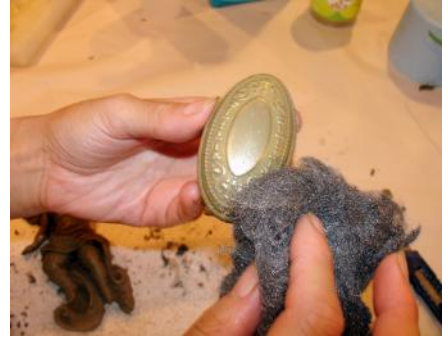
Step 16. Once the cast was set we removed the cast knob and polished with 000 steel wool to expose the brass surface.
