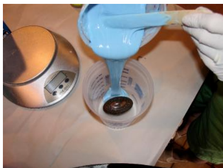
Step 7. After mixing well, we poured into the mold container in a long narrow stream. We poured in one spot letting the rubber envelope the knob. This drives out more air.
