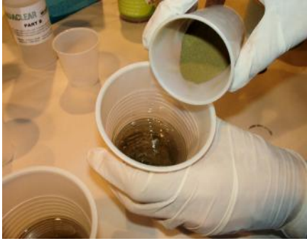
Step 14. We added half the brass powder to Part A and the balance to Part B and stirred well.
