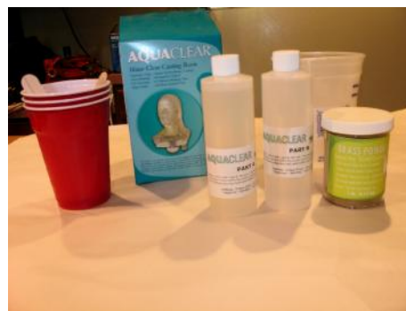
Step 11. To create a brass casting these we needed 325 Mesh brass powder and AquaClear resin along with some cups and mixing sticks.
