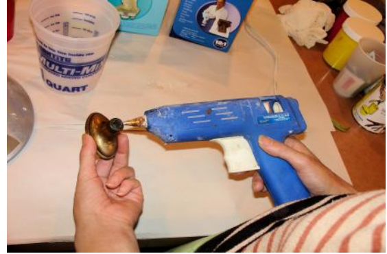
Step 2. We placed a small dab of hot glue on the bottom of our part.
