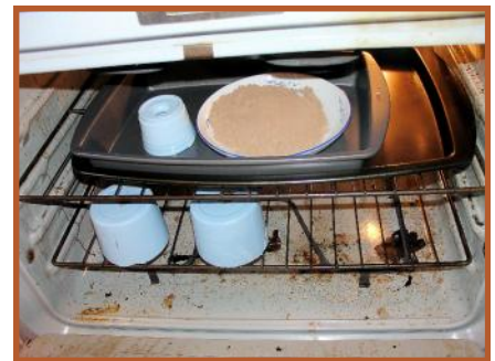
The pecan shell powder is dried in the oven along with a number of molds.
