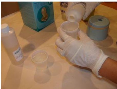
Step 12. We measured out equal parts of Part A and Part B in two cups.
